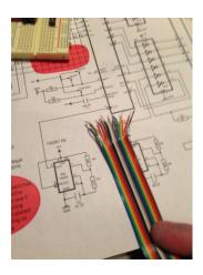
The most difficult task of the Datanetics keyboard build is to create the cable to connect the keyboard to the Apple-1. Using a rainbow 16 wire ribbon cable makes the implementation easier to keep track of.
