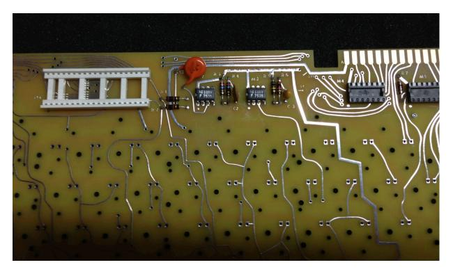
Installing the soldered components is the easiest part of the keyboard build. You will not install the key switches at this point, but all other components will be installed.
