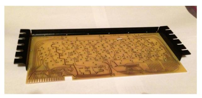
After initially attaching the sides, drill the rest of the holes and use eyelets to attach.
