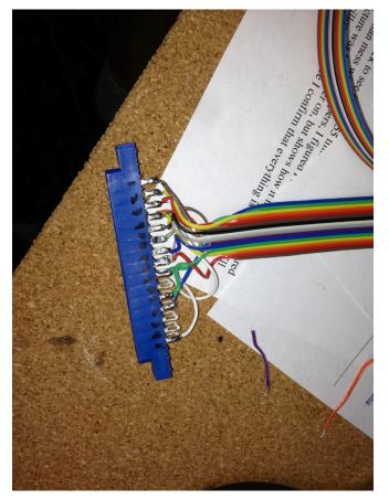
To build the cable you will need to first separate using a sharp knife blade the individual wires on one side of the cable. You will need to go back about 6" into the cable to give you enough room to make clean connections. If you are comfortable building the cable (i.e. this isn't your first) you may go shorter.
