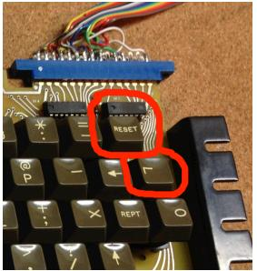
After clearing screen and resetting, Go through the keyboard shorting each pair of pads making sure that each key works, than as in the picture below, jumper the shift key and checked that shift characters work (i.e. numeric keys). You may also with to test the repeat function.
