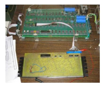
To initially test your keyboard, plug in the MM5740 and the two 7404s. You will need to check for hot chips.
