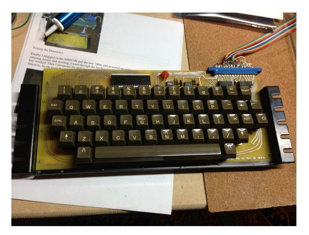
Follow the pattern above to install the key caps. To install the space bar, there are two hinge brackets for the spacer's metal torsion bar. You may need to adjust which hole the bar goes though.
