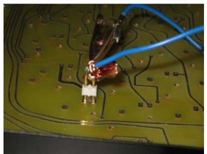
If you get strange results, you need to check that you do not have partial connections in the matrix that was drilled or reamed out. Remember to use an ohm meter and not a continuity tester.
